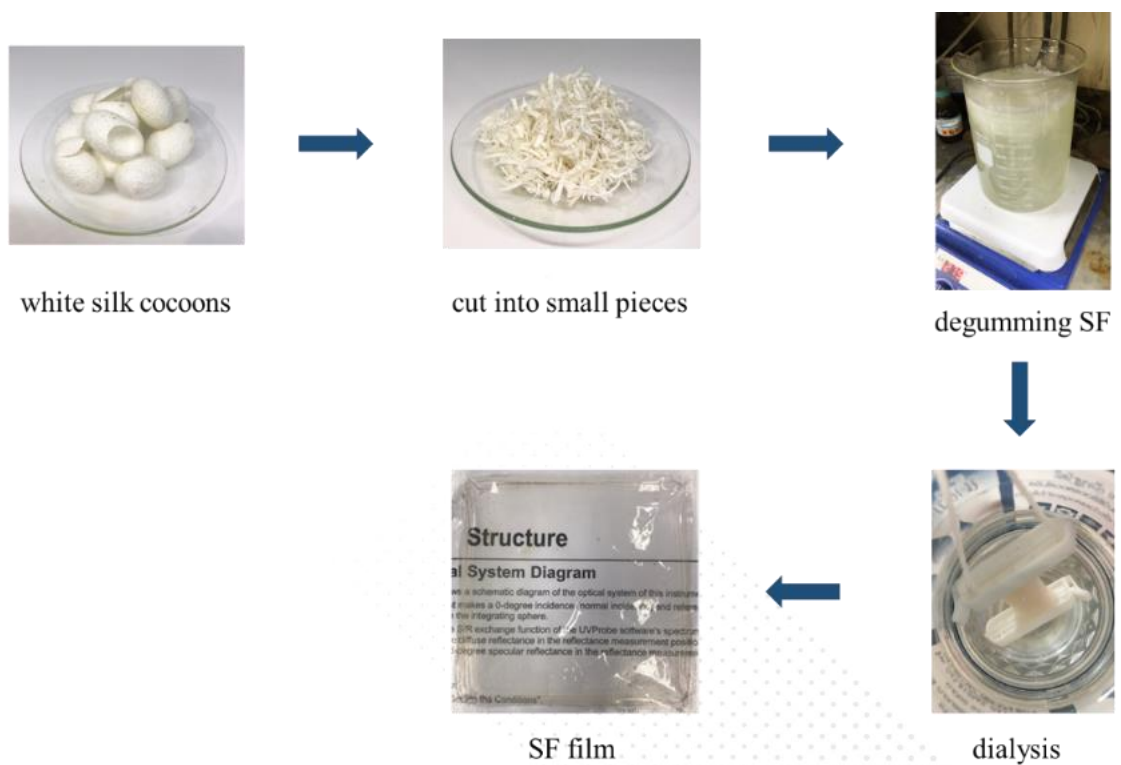
Figure 1. Sequence steps in preparation of silk fibroin film.
