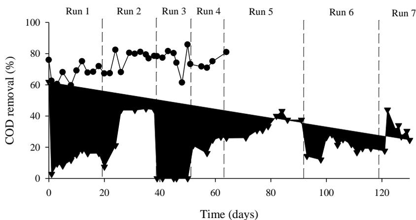
**Fig. 1** Effect of isothiazolone on COD removal in the RBCs: control (●) and 6 ppm (▼). (The operating conditions in Run 3 and Run 4 of the control RBC were identical).
