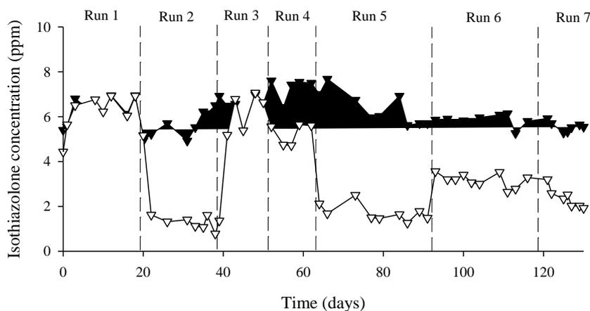
**Figure 2** Isothiazolone removal in the RBCs: influent (▼), effluent (▽).
